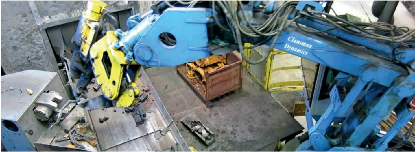
PB20 working with C2010 manipulator mounted with CC112 degating hammer
