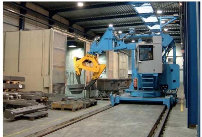
C5010 rail bond manipulator with 5 tons capacity
