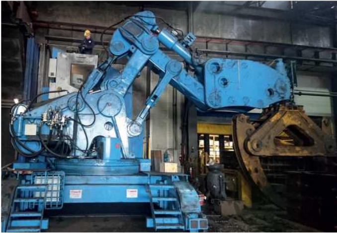
C20020 rail bound manipulator with 20 tonnes capacity
