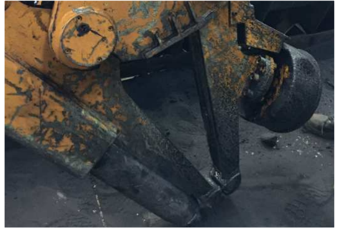
Gripper with cannon and magnet
