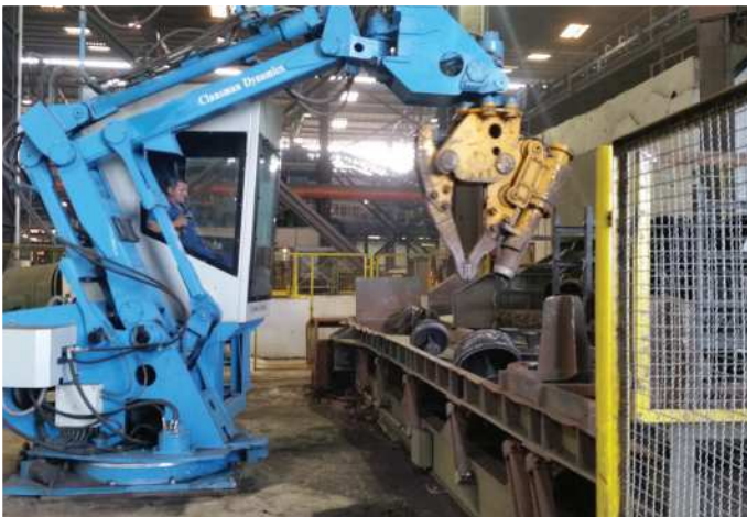
C620 manipulator with gripper mounted cannon
